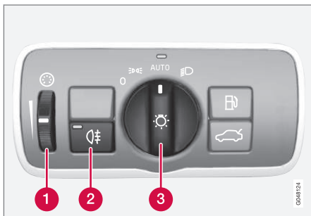
Lighting panel overview
