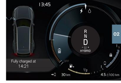
Indicates that the Charge or Hold functions are active. These are activated from the center display's Function view. Charge means that the hybrid battery is being charged if its charge level is low. Hold means that the battery level is being retained for later use.
