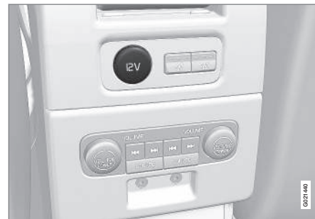
12 V socket in tunnel console, rear seat.
