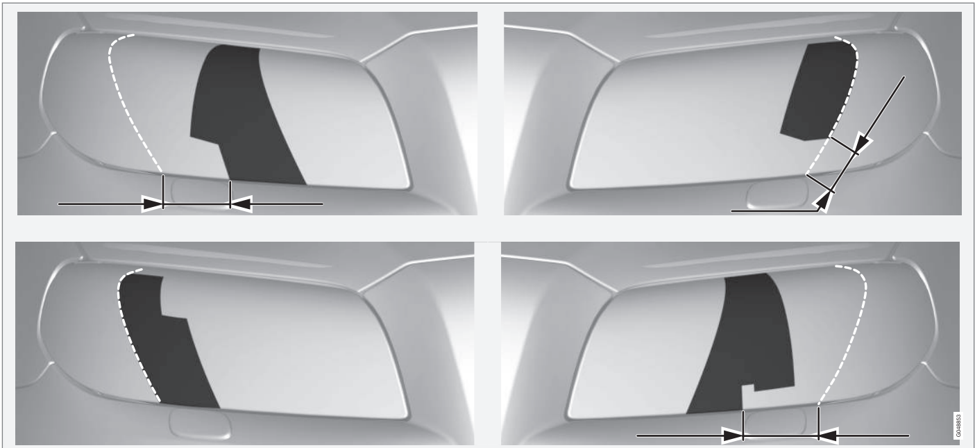
Upper row: left-hand drive cars, templates A and B. Lower row: right-hand drive cars, templates C and D.
