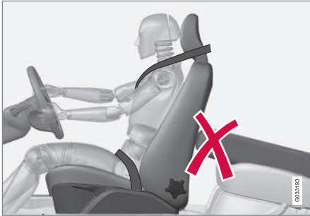
Do not place objects on the rear seat that may prevent the WHIPS system from functioning.
