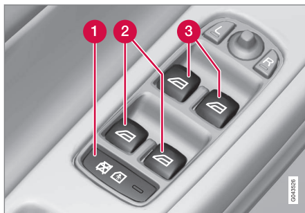
Driver's door control panel.
