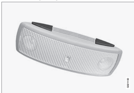
Rear roof lighting.
