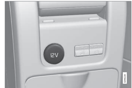
12 V socket in tunnel console, rear seat.
