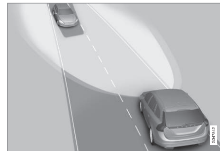
Adaptive functionality: Dipped beam directly toward oncoming vehicles, but continued main beam on both sides of the vehicle.
