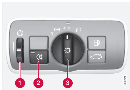
Lighting panel overview
