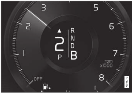
Gear shift indicator in the driver display 5 .
