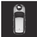
A camera symbol on the centre display's car symbol indicates which of the cameras is active.
