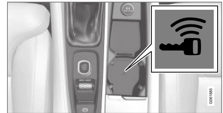
Backup reader's location in the tunnel console.
