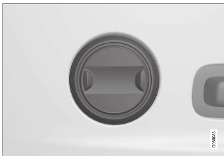
Control in cars with two-way lumbar support*.
