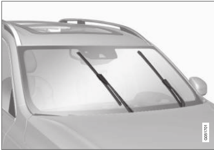
Wiper blades in service position.
