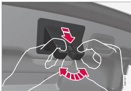
Rubber casing over the boot lid lock.
