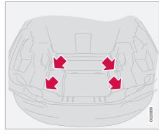
There are four or more eyelets for securing straps or ropes. Straps that are suitable for the eyelets are supplied by Volvo dealers.
