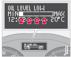
The figures 1-4 represent filling level. Do not fill more oil if filling level (3) or (4) is shown. Recommended filling level is 4.
