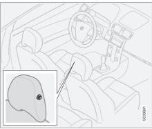
The coat hanger is located on the passenger seat head restraint. Only hang light garments on the hanger.
