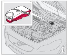
Brake and clutch fluid have a common reservoir<sup>4</sup>. The fluid level must be between the **MIN** and **MAX** marks. Check the level regularly. Change the brake fluid every other year or at every other regular service.
