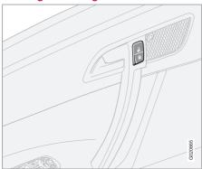
With the central locking buttons on the doors, the doors and boot lid can be locked or unlocked simultaneously.
