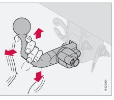
7. Check that the towbar is secure by pulling it up, down and back.
