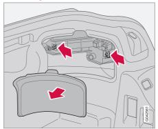
All bulbs in the rear lamp cluster can be replaced from inside the cargo area.
