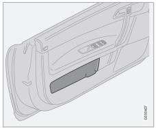
The storage compartment is opened by lifting the lower front edge of the lid, and closed with a touch on its upper section.
