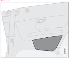
The storage compartment is opened and closed with a touch in the centre of its upper section.
