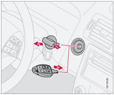
If the remote control key's battery is discharged then the Keyless Drive function does not work. In which case, start the car by using the remote control key as ignition dial.
