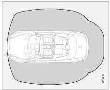
The keyless drive system allows the car to be unlocked, driven and locked without the need for a key. You simply need to have the remote control key with you in a pocket or a bag.
