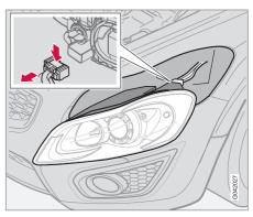
5. Lift out the lamp housing and place it on a soft surface to avoid scratching the lens.
