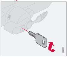
Insert the key and turn it clockwise to the unlocked position.
