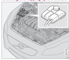
When topping up the coolant, follow the instructions on the packaging. It is important that the mixture of coolant concentrate and water is correct for the prevailing weather conditions. Never top up with water only. The risk of freezing increases with both too little and too much coolant concentrate.
