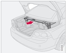
The purpose of the separator is to limit the amount of the load in the cargo area so that the movement of the roof is not disrupted. Be sure to close the cargo separator fully so that it is locked on both the left and right-hand sides.
