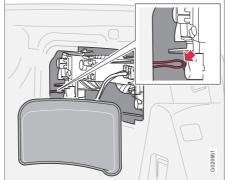
Manual opening of the fuel filler flap is easier when the roof is closed, and is used when it is not possible to open it from the passenger compartment.
