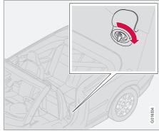
If the car's electrical systems are temporarily out of order then the boot lid can be opened mechanically with the remote control key's detachable key blade. For information on removing the key blade, see page 121.
