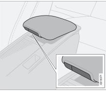
There is a storage space under the armrest. There is also a smaller storage space in the detachable armrest. Press the small button and lift the armrest to open the shallow compartment. Press the large button and lift the armrest to open the deeper compartment.
