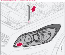
All front bulbs (except for fog lamps) are changed by first removing the lamp housing from the engine compartment.
