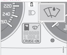
The rain sensor automatically activates the windscreen wipers based on how much water it detects on the windscreen. The sensitivity of the rain sensor can be adjusted using the thumbwheel (2), see page 65.
