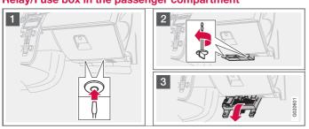
The fuse box has 50 fuse positions. The fuses are located under the glovebox. The box also provides space for several spare fuses. Tools for fuse replacement are located in the relay/ fuse box in the engine compartment, see page 228.
