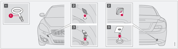
The towing eye is screwed into a threaded socket behind a cover on the right-hand side of the bumper, front or rear.
