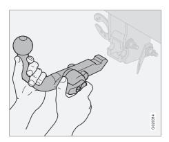
Turn the locking wheel down fully, until it comes to a stop. Hold it in this position while pulling the towbar rearward and upward.
