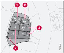
When the phone is active, the steering wheel keypad is locked to phone functions. To control the audio system, the phone must be in standby mode (standby).
