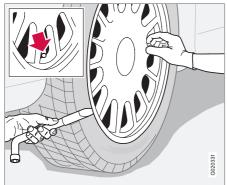
Set up the warning triangle if a wheel must be changed at a busy location. Make sure that the car and jack are on a firm horizontal surface.
