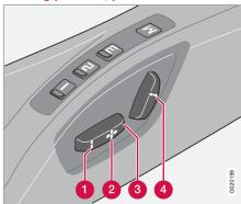
The seats can be adjusted for a certain time after unlocking the door with the remote control key without the key being inserted into the ignition switch. The seat can always be adjusted in key position I or II.
