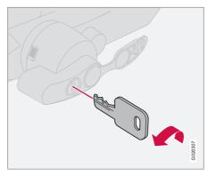
6. Turn the key anticlockwise to locked position. Remove the key from the lock.
