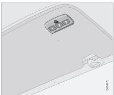
HomeLink<sup>®1</sup> is a programmable remote control which can remotely control up to three different devices (e.g. garage door opener, alarm system, outdoor lighting and indoor lighting etc.) and in doing so replace their remote controls. For more information on HomeLink<sup>®</sup>, visit: www.homelink.com or ring 00 8000 466 354 65 (or premium rate phone number, +49 6838 907 277).
