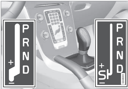
D: Automatic gear positions. +/–: Manual gear positions. S: Sport mode*. 6
