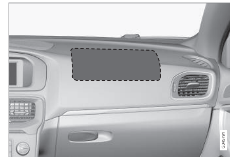
Location of the front passenger airbag in a left-hand drive car.
