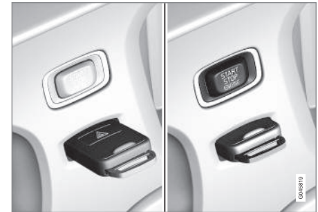
Ignition switch with remote control key extracted/inserted.
