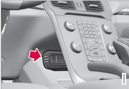
Handheld unit storage and charging station.
