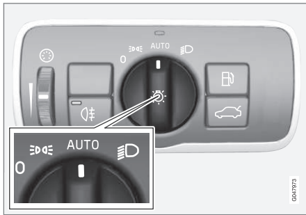
Knob for headlamp control in AUTO position.
