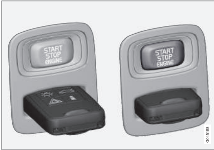
Ignition switch with remote control key extracted/inserted.
