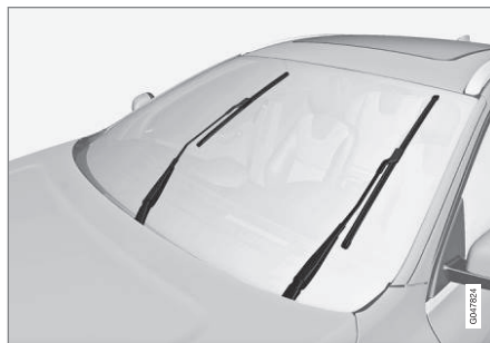
Wiper blades in service position.
