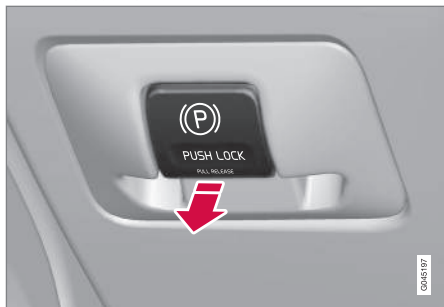
Parking brake control - release.
