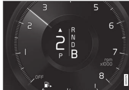
Gear shift indicator in the driver display 5 .
