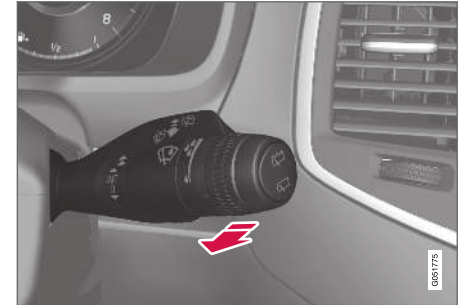
Washing function, right-hand stalk switch.
