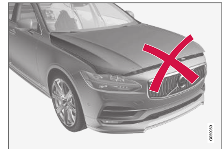
Bonnet not completely closed.
