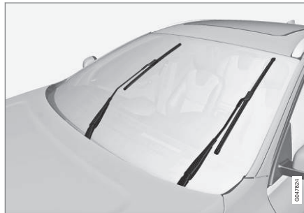
Wiper blades in service position
