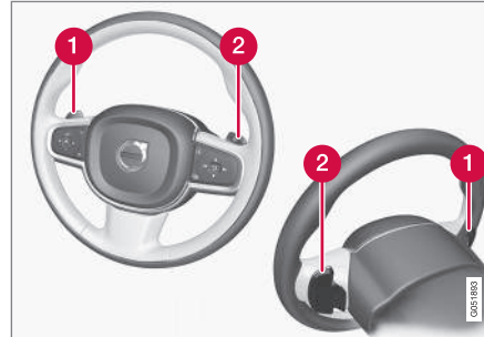
Instrument panel when shifting gears using steering wheel paddles, large gear selector.
