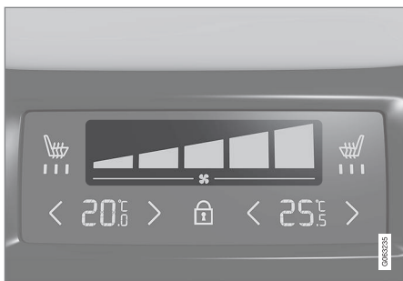
Blower controls on the rear climate panel of the tunnel console.
