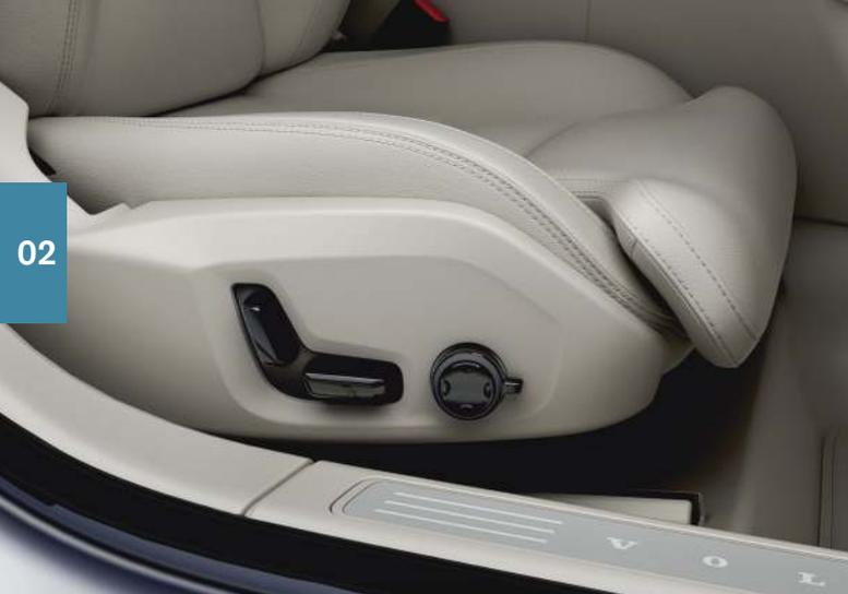
2. Switch between the various functions in the center display by turning the control upward/downward.
