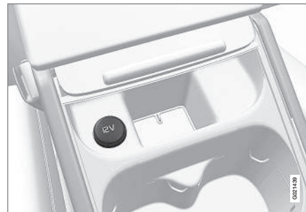
12 V socket in tunnel console, front seat.
