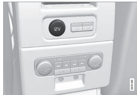
12 V socket in tunnel console, rear seat.
