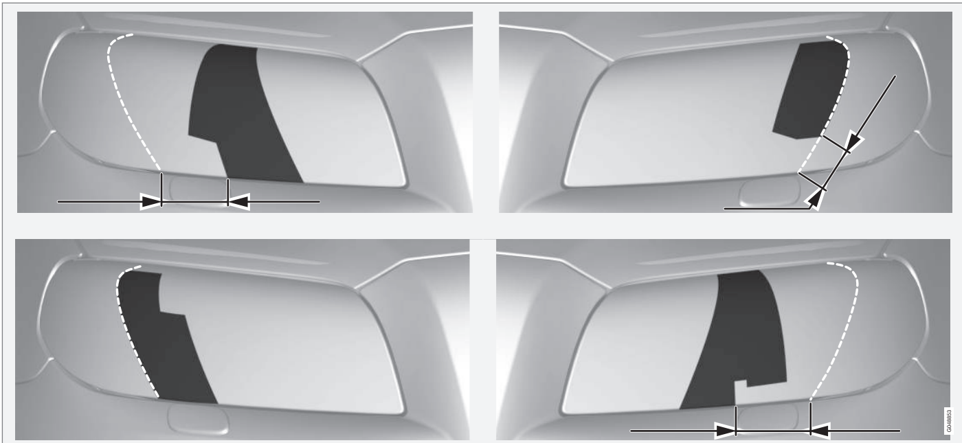
Upper row: left-hand drive cars, templates A and B. Lower row: right-hand drive cars, templates C and D.
