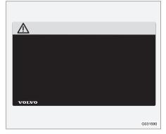
Black ISO symbols on yellow warning field, white text/image on black message field. Used to indicate the presence of danger which, if the warning
