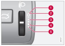
Thumbwheel positions for different load cases.
