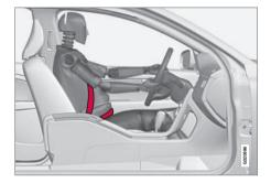
The diagonal section should wrap over the shoulder then be routed between the breasts and to the side of the abdomen.
