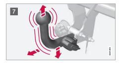
Check that the towball section is secure by pulling it up, down and back.
