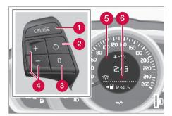
The steering wheel buttons and display in cars  $\mbox{\it without}$  speed limiter  $^{7}.$
