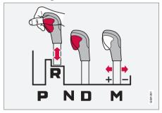
The gear selector can be moved forward and back freely between  $\bf N$  and  $\bf D$ . Other positions are locked with a latch that is released with the inhibitor button on the gear selector.
