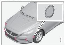
The PAP sensors are located in the bumpers<sup>44</sup> - 6 front and 4 rear.
