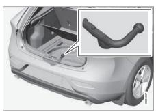
The detachable towbar must be stored in the foam block<sup>14</sup> under the cargo area floor when not in use.
