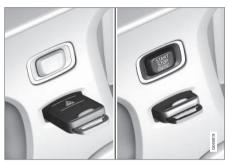
Ignition switch with remote control key extracted/inserted.
