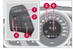
The steering wheel buttons and display in cars **without** speed limiter<sup>3</sup>.
