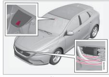
Camera and radar sensor<sup>24</sup>.
