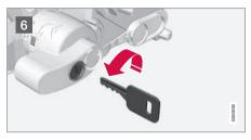
Turn the key anticlockwise to locked position. Remove the key from the lock.
