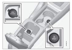
12 V socket in tunnel console, front seat,
