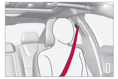
Correctly fitted seatbelt.
