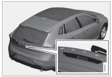
Rubber plate with electrical contact.
