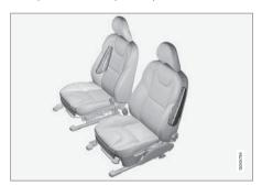
The SIPS bag system consists of two main components, side airbag and sensors. The side airbags are located in the front seat's backrests.
