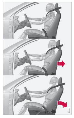
The WHIPS system is actuated by a rear-end collision, where the angle and speed of the collision,
