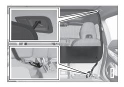
Hook the hooks into the roof mounting with the anchoring strap locks turned towards you.
