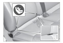
Mounting points for the ISOFIX fixture system are located at the lower section of the rear seat backrest, in the outer seats.
