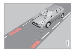
A camera reads the painted side lines of the road/lane. If the car is about to cross a side line then Lane Keeping Aid will actively steer the car back into the lane with a slight steering torque in the steering wheel.
