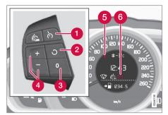
The steering wheel buttons and display in cars **with** speed limiter<sup>7</sup>.
