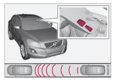
Laser sensor transmitter and receiver window<sup>16</sup>.
