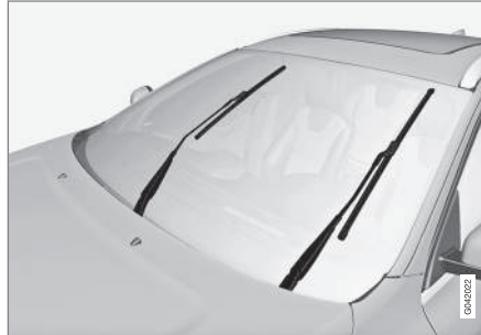
Viskerblade i servicestilling.
