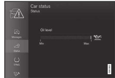
Graphics for oil level in the centre display.
