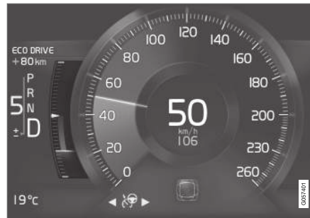
Eco gauge in the 8-inch driver display.
