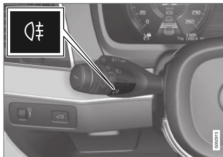
Button for rear fog lamp.
