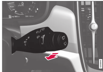
Washing function, right-hand stalk switch.
