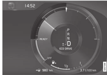
Eco gauge in the 12-inch driver display*.
