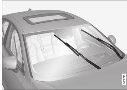
Wiper blades in service position.
