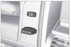
Ianition switch with inserted remote control key and START/STOP ENGINE button.
