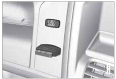
Ignition switch with inserted remote control key.
