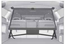
The safety net is fitted into four mounting points.
