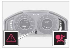
The warning symbol in the combined instrument panel illuminates when the remote control key is in key position II or III. The symbol clears after approx. 6 seconds provided the airbag system is fault-free.
