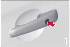
Cars with the keyless system have a button on the outside door handles.
