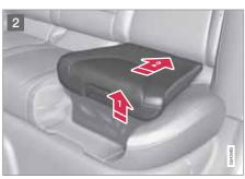
2 Lift the booster cushion up at the front edge and press it back against the backrest to lock.
