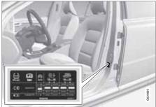
The tyre pressure decal on the driver's side door pillar (between frame and rear door) shows which pressures the tyres should have at different loads and speed conditions. This is also specified in the tyre pressure table, see page 304.
