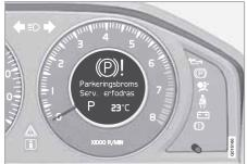
Park brake not fully released - A fault is preventing the parking brake from being released. Visit a workshop - an authorised Volvo workshop is recommended. A warning signal sounds if you pull away with this error message.
