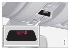
Unbelted occupants will be reminded to fasten their seatbelts by means of an audio and visual reminder. The audio reminder is speed dependent, and in some cases time dependent. The visual reminder is located in the roof console and the combined instrument panel.
