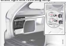
Both the brake light and the reversing lamp bulbs are replaced from inside the cargo area.
