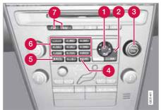
Centre console, controls for radio functions.
