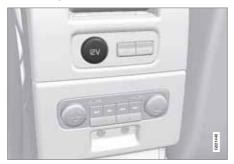
12 V socket in tunnel console, rear seat.
