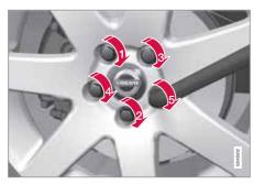
Tighten the wheel bolts crosswise. It is important that the wheel bolts are tightened properly. Tighten to 140 Nm. Check the torque with a torque wrench.
