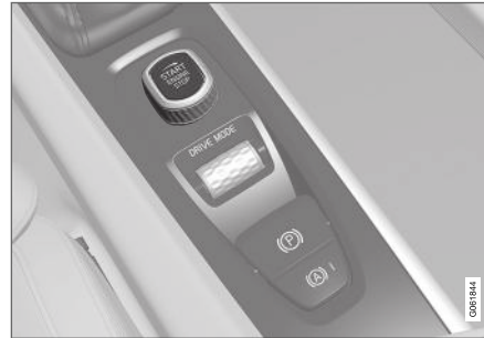
Start knob in the tunnel console.
