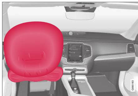
Steering wheel airbag and knee airbag on the driver's side in the front seat.
