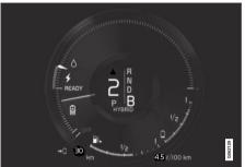
The car generates current to the battery and the battery is charged, e.g. when the brake pedal is pressed gently or during engine braking down a hill.
