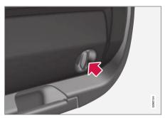
Detach the panel on the inside of the tailgate by first turning the two knobs a quarter turn anticlockwise and then unhooking the panel. Place the panel to one side.
