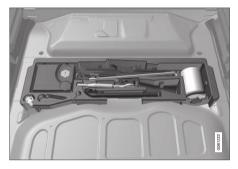
The foam block under the cargo area floor contains the car's towing eye, puncture repair kit, tool for removing the plastic caps from the wheel bolts and a socket for the lockable wheel bolts.
