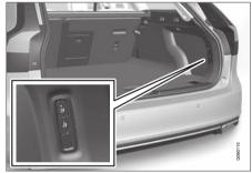
To facilitate folding of the rear seat, the car must be stationary and the tailgate open. Ensure that there are no occupants or objects in the rear seat.
