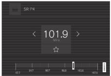
On changing over to manual tuning, the radio no longer changes frequency automatically when reception is poor.
