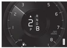
Gear shift indicator in the driver display<sup>3</sup>.
