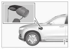
Charging cable handle and charging input socket.
