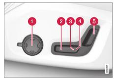
The illustration shows the controls from a car with fourway lumbar support\*. Cars with two-way lumbar support\* do not have the rotatable multifunction control.
