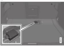
Fit a personal SIM card into the holder under the cargo area floor.
