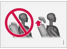
The centre seat's head restraint must be adjusted according to the passenger's height so that, if possible, the whole of the back of the head is covered. Slide it up manually as required.
