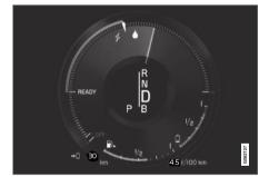
The electric motor cannot supply the amount of engine power requested and the internal combustion engine starts.
