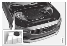
Coolant expansion tank, left-hand drive car.
