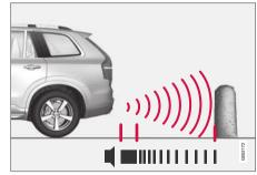
Warning signal, constant tone at less than approx. 30 cm (1 ft) from an obstacle <sup>110</sup>.
