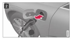
Unplug the cable from the car's charging input socket and close the hatch.
