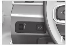
Thumbwheel (to left) for adjusting interior brightness.
