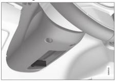
Lever for steering wheel adjustment.
