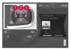
Message in the driver display and the steering wheel's right-hand keypad.
