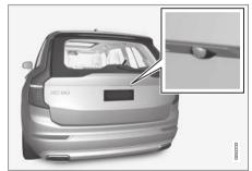
The backwards-facing camera  $^{115}$  is fitted above the registration plate.
