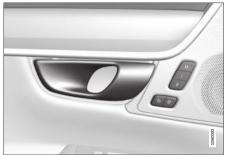
Opening handle for alternative unlocking in the side  $door^{15}$ .
