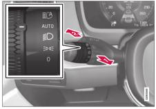
Steering wheel stalk switch with rotating ring.
