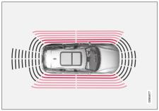
Warning signal, intensive pulsing at less than approx. 25 cm (0.8 ft) from an obstacle <sup>110</sup>.
