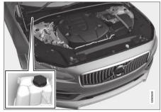
Coolant expansion tank, right-hand drive car.
