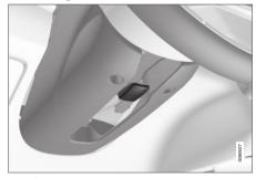
Lever for steering wheel adjustment.
