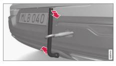
Screw the eye in firmly. For example, thread through the wheel bolt wrench\* and use it as a lever.
