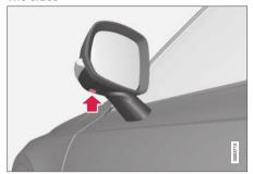
The side cameras 116 are positioned in each door mirror.
