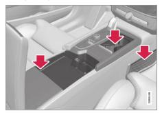
Storage spaces with cup holder, electrical socket, mesh pocket\* and USB port in the tunnel console.
