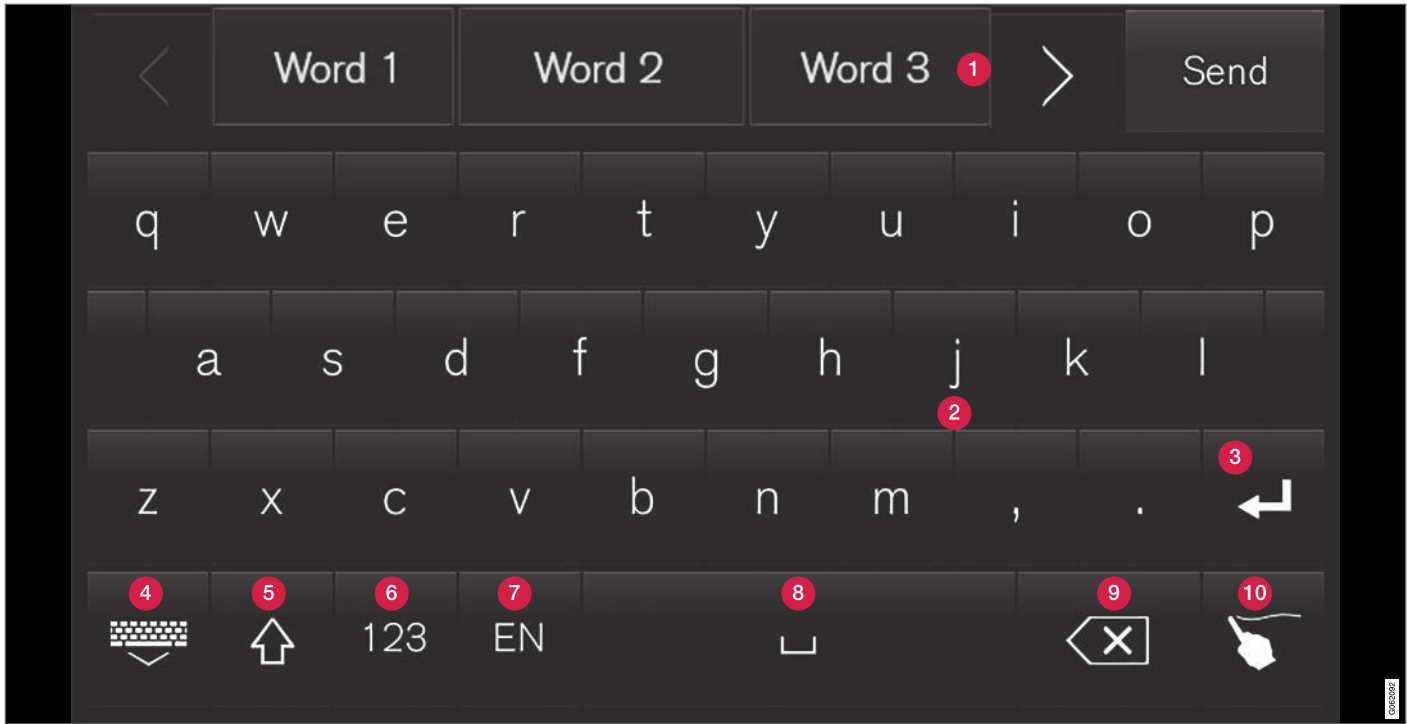
The illustration shows an overview of some of the buttons that may be shown on the keyboard. The appearance may vary depending on language settings and the context in which the keyboard is used.
