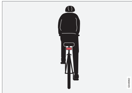
Optimal example of what the system interprets as a cyclist - with clear body and bicycle contours, directly from behind and in the car's centre line.
