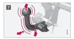
Check that the towbar is secure by pulling it up, down and back.
