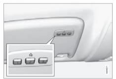
HomeLink®¹ is a programmable remote control which can remotely control up to three different devices (e.g. garage door opener, alarm system, outdoor lighting and indoor lighting etc.) and in doing so replace their remote controls. For more information on HomeLink®, visit: www.homelink.com or ring 00 8000 466 354 65 (or premium rate phone number, +49 6838 907 277).
