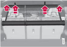
Pull the net up from the cassettes. The net is self-locking after about 1 minute if the rear seat's backrests are raised.
