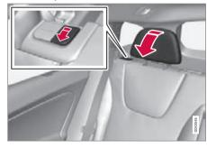
Pull the locking handle closest to the head restraint to fold the head restraint forward.
