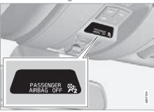
Indicator showing that the passenger airbag is deactivated.
