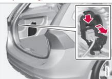
The bulbs for reversing lamp, fog lamp and direction indicator in the rear lamp cluster are replaced from inside the cargo area.
