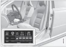
The tyre pressure decal on the driver's side door pillar (between frame and rear door) shows which pressures the tyres should have at different loads and speed conditions. This is also specified in the tyre pressure table, see page 408.
