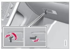
The glovebox can only be locked/unlocked using the remote control key's detachable key blade. For information on the key blade. see page 48.
