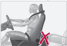
Do not leave any objects on the floor behind the driver's seat/passenger seat that may prevent the WHIPS system from functioning.
