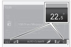
Current temperature for each side is shown in the centre console's screen.
