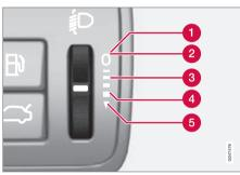
Thumbwheel positions for different load cases.
