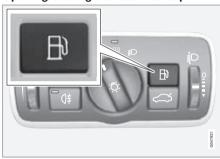
Open the fuel filler flap using the button on the lighting panel - the flap opens when the button is released.
