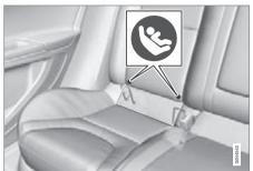
Mounting points for the ISOFIX fixture system are concealed behind the lower section of the rear seat backrest. in the outer seats.
