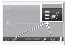
Current heat level is shown in the centre console's screen.
