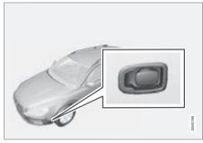
Electrical input to the engine block heater.
