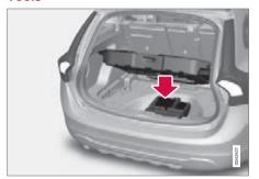
Located under the cargo area floor are the car's towing eye, jack\* and wheel wrench\*. There is also space for the sleeve for the lockable wheel bolts.
