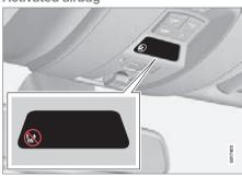
Indicator showing that the passenger airbag is activated.
