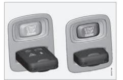
Ignition switch with remote control key extracted/inserted
