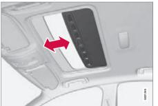
One long press on the lock button closes the sunroof and all the windows, see pages 45 and 59. The doors and the tailgate are locked. To interrupt closing, press the lock button again.
