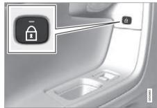
The button's lamp illuminates when the door is locked.
