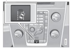
The function is switched on or off by means of a button on the centre console. An indicator lamp in the button illuminates when the function is switched on.
