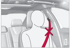
Incorrectly fitted seatbelt. The belt must rest on the shoulder.
