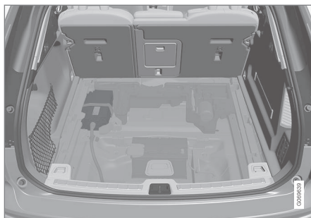
If the car is equipped with a 48V support battery instead, it is located on the left in the cargo area. The 48V support battery must only be handled by an authorised workshop.
