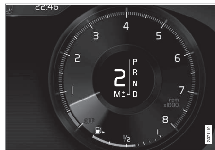
Driver display when changing gear with steering wheel paddles in manual gearshift mode, large gear lever.
