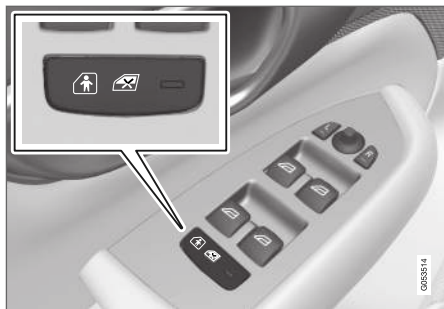
Button for electric activation and deactivation.
