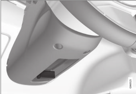
Lever for steering wheel adjustment.
