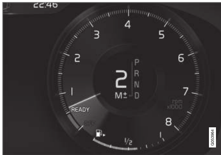
manual gearshift mode in the driver display 3 .
