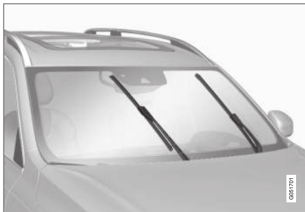
Wiper blades in service position.
