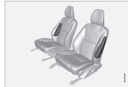
Location of the side impact (SIPS) airbags (front seats only)
