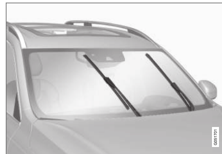
Viskerblade i servicestilling.
