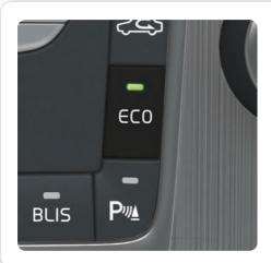
One press on **ECO** activates an optimal fuel-efficient driving program including, amongst other things, the following changes:
