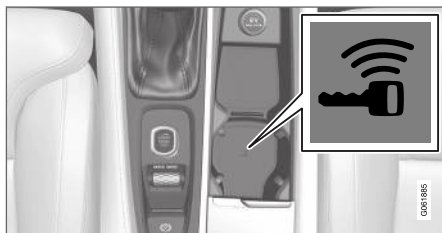
Backup reader's location in the tunnel console.
