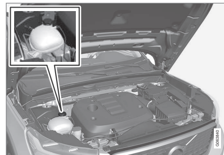
Coolant expansion tank.
