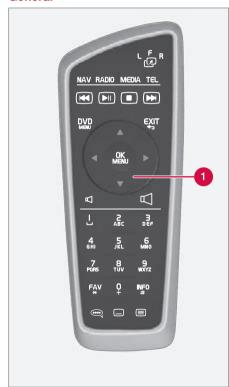
The remote control can be used for all functions in the infotainment system. The remote control's buttons have the same functions as the buttons in the centre console or steering wheel keypad\*.
