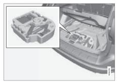
Emergency puncture repair (TMK; Temporary Mobility Kit)<sup>1</sup> is used to seal a puncture and check and adjust tyre pressure. It consists of a compressor and a bottle with sealing fluid. The kit works as a temporary repair. The sealing fluid bottle must be replaced before its expiration date and after use.
