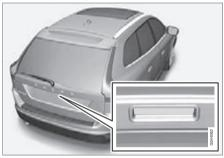
Rubber plate with electrical contact.
