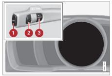
Information display (digital combined instrument panel) and controls for menu navigation.
