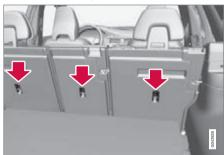
The car is equipped with upper mounting points for certain front-facing child seats. These mounting points are located on the rear of the seat.
