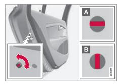
The child safety locks are located on the trailing edge of the rear doors and are only accessible when the doors are open.
