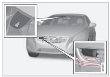
Camera and radar sensor<sup>3</sup>.
