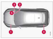
Central electrical unit locations in a left-hand drive car. In a right-hand drive car the central electrical units under the glovebox change sides.
