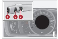
Information display (analogue combined instrument panel) and controls for menu navigation.
