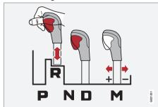
The gear selector can be moved forward and back freely between **N** and **D**. Other positions are locked with a latch that is released with the inhibitor button on the gear selector.
