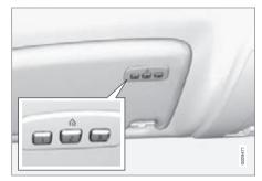
HomeLink<sup>®1</sup> is a programmable remote control which can remotely control up to three different devices (e.g. garage door opener, alarm system, outdoor lighting and indoor lighting etc.) and in doing so replace their remote controls. For more information on HomeLink<sup>®</sup>, visit: www.homelink.com or ring 00 8000 466 354 65 (or premium rate phone number, +49 6838 907 277).
