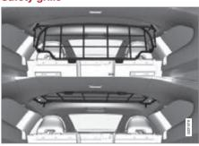
A safety grille prevents loads or pets from being thrown forward in the passenger compartment in the event of sudden braking.
