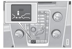
Press the button in the centre console to switch the function on or off. The function is switched on if one lamp is illuminated in the button.
