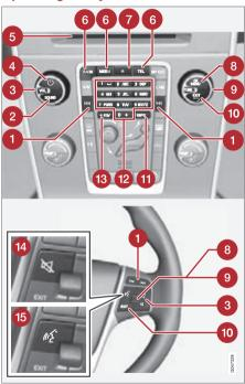
① Scroll/fast wind/search - short press scrolls between disc tracks, preset radio stations (does not apply to DAB) or chapter (only
