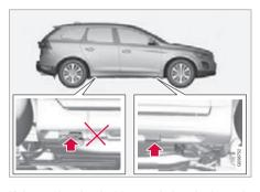
If the car is raised with a workshop jack; position the jack against the front edge on the engine's subframe.
