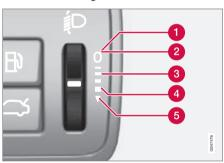
Thumbwheel positions for different load cases.
