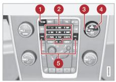
Centre console, controls for radio functions.
