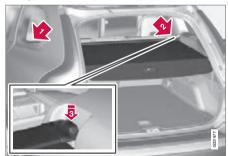
Pull the cargo cover over the load and hook it into the recesses at the cargo area's rear posts.
