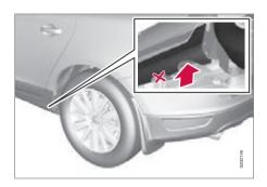
Check that the jack sits in the anchorage as illustrated and that the foot is positioned vertically under the anchorage.
