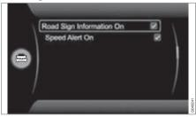
The combined instrument panel's speed symbol display can be disabled. To deactivate the RSI function:
