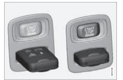
Ignition switch with remote control key extracted/inserted.
