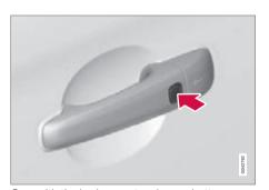
Cars with the keyless system have a button on the outside door handles.
