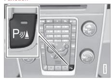
The system is automatically activated when the engine is started - the switch's On/Off lamp is illuminated. If parking assistance is switched off with the button, the lamp goes out.
