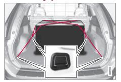
The folding load retaining eyelets are used to fasten straps in order to anchor items in the cargo area.
