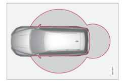
The keyless drive function in the PCC allows the car to be unlocked, driven and locked without the need for a key. You simply have to have the PCC with you. The system makes it easier and more convenient to open the car, e.g. when your hands are full.
