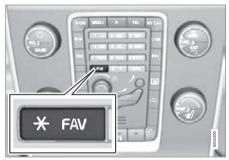
The **FAV** button can be used to store functions that are used frequently so that the function can be started simply by pressing **FAV**. You can select a favourite (e.g. **Equalizer**) for each function as follows:
