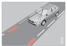
The LDW (Lane Departure Warning) function is intended to reduce the risk of so-called single-vehicle accidents – accidents where, in certain situations, the vehicle leaves the carriageway and is in danger of driving either into a ditch or into oncoming traffic.
