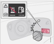
Don not forget to switch off the fuel-driven heater before refuelling!
