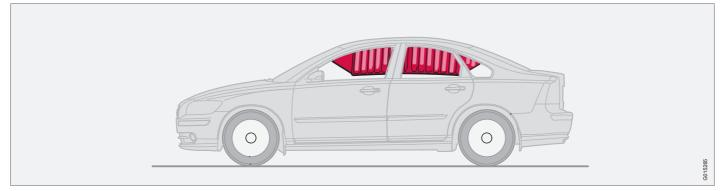
The inflatable curtain IC (Inflatable Curtain) is a part of SIPS and the airbags. It is fitted in the headlining along both sides of the roof and protects the car's occupants sitting in the outer seats. A sufficiently violent collision trips the sensors and the inflatable curtain is inflated. The inflatable curtain helps to prevent the driver and passengers from striking their heads on the inside of the car during a collision.
