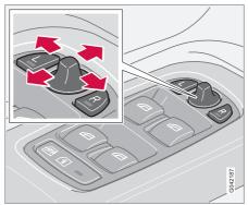
The controls for adjusting the two door mirrors are at the front of the driver's door armrest. The rearview mirrors can be operated in key position  ${\bf I}$  and  ${\bf II}$ .
