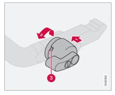
3. Check that the indicator window (3) shows red. If the window does not show red, press in 1 and turn the locking wheel anticlockwise 2 until you hear a click.
