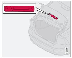
The warning triangle is fitted on the inside of the boot lid with two clips.
