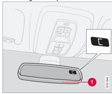
The earth is divided into 15 magnetic zones. The compass is set for the geographical area to which the car was delivered. The compass should be calibrated if the car is moved across several magnetic zones.
