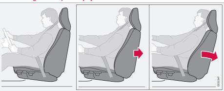
The whiplash protection system (WHIPS) consists of energy absorbing backrests and specially designed head restraints for the front seats. The system is actuated by a rear-end collision, where the angle and speed of the collision, and the nature of the colliding vehicle all have an influence.
