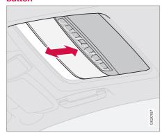
One long press on the lock button closes the sunroof and all the windows. The doors and the boot lid are locked. If you need to interrupt closing:
