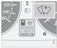
The rain sensor automatically activates the windscreen wipers based on how much water it detects on the windscreen. The sensitivity of the rain sensor can be adjusted using the thumbwheel (C), see page 67.
