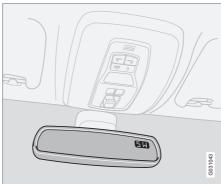
The upper right-hand corner of the rearview mirror has an integrated display that shows the compass direction in which the front of the car is pointing. Eight different directions are shown with English abbreviations: N (north), NE (north east), E (east), SE (south east), S (south), SW (south west), W (west) and NW (north west).
