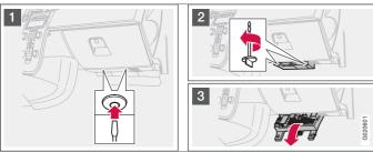
The fuse box has 50 fuse positions. The fuses are located under the glovebox. The box also provides space for several spare fuses. Tools for fuse replacement are located in the relay/fuse box in the engine compartment, see page 236.
