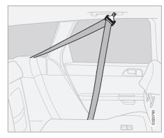
The rear seat backrests can be tipped forwards together, or individually, to make it easier to transport long objects. To avoid damaging the seatbelts when folding the backrests up or down, these should be hooked onto the grab handles.
