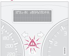
If the car is involved in a collision, the text CRASH MODE SEE MANUAL may appear on the information display. This means that the car has reduced functionality. Crash mode is a protective state that is enforced when the collision may have damaged any of the car's vital functions, such as the fuel lines, sensors for one of the safety systems, or the brake system.
