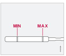
The oil level must be within the area marked on the dipstick.
