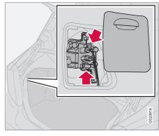
All bulbs in the rear lamp cluster are replaced from inside the cargo area.
