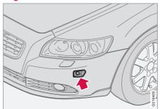
Electrical input to the engine block heater.
