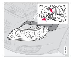
5. Lift out the lamp housing and place it on a soft surface to avoid scratching the lens.
