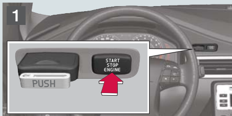
Park the car and press the START/STOP/ENGINE button to switch off the engine.
