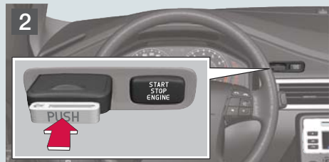
Press gently on the remote key, which is then pushed out. Automatic transmission must be in position P .
