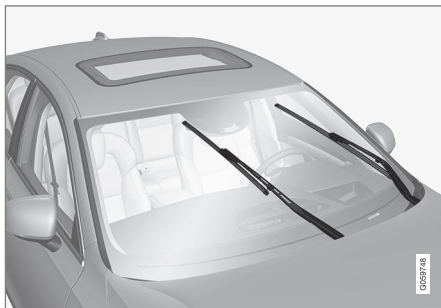
Viskerblader i servicestilling.
