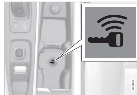
Backup reader's location in the tunnel console.
