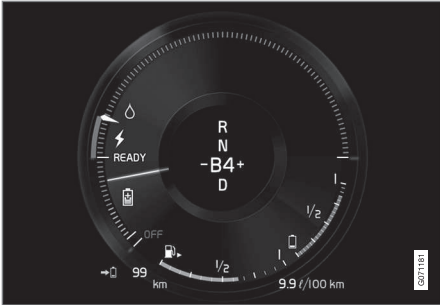
The driver display indicates charging during electric motor braking. This function is active in the speed interval 150-5 km/h (93-3 mph). During heavier brak-
