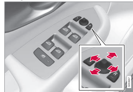
Controls for door mirrors.
