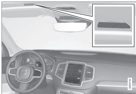
Voice control system microphone
