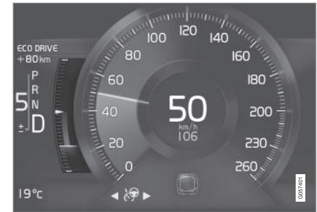
Eco gauge in the 8-inch driver display.
