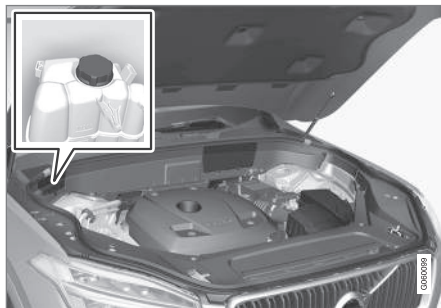
Coolant expansion tank.
