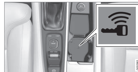
Backup reader's location in the tunnel console.
