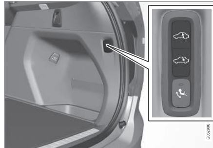
Controls for raising/lowering the car's rear section.
