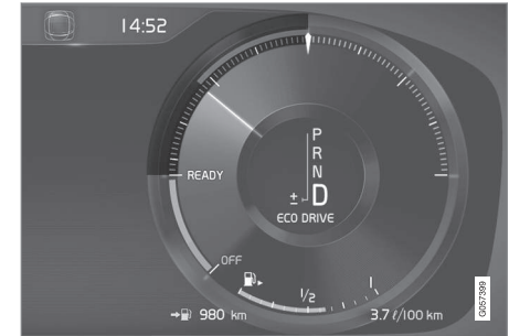
Eco gauge in the 12-inch driver display.
