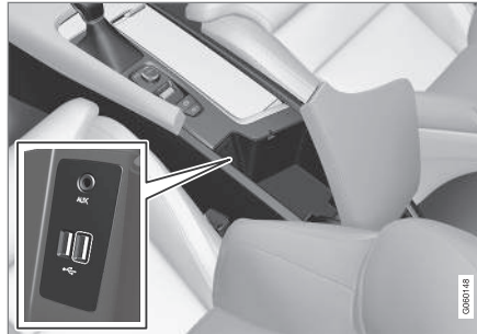
USB socket in tunnel console.
