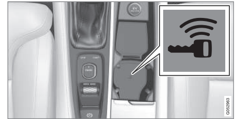
Backup reader's location in the tunnel console.
