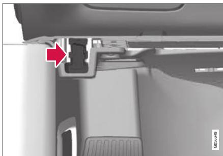
Prise de diagnostic (prise On-board Diagnostic, OBDII)
