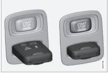
Ignition slot with remote key and START/STOP ENGINE button.
