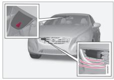
Camera and radar sensor<sup>5</sup>.
