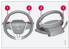
Steering-wheel mounted gear shift paddles
