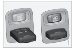
Ignition slot with remote key inserted (see Ignition modes (p. 69) for more information on ignition modes)
