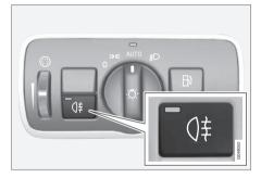
The rear fog lights will only function in combination with the high/low beam headlights.
