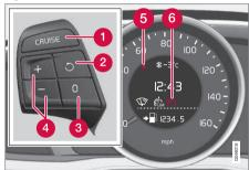
Steering wheel-mounted controls and display
