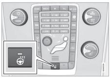
Button for steering wheel heating
