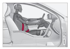
The diagonal section should wrap over the shoulder then be routed between the breasts and to the side of the belly. The lap section should lay flat over the thighs and as low as possible under the belly. It must never be allowed to ride upward. Remove all slack from the belt and ensure that it fits close to the body without any twists.
