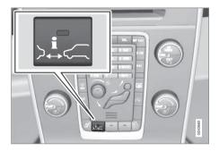
Press the button in the center instrument panel to switch this function on or off. The indicator light in the button illuminates when the function is on.
