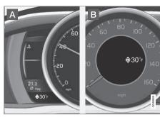
Location of the ambient temperature sensor, A: digital instrument panel\*, B: analog instrument panel
