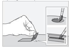
Place a strip of masking tape over the damaged surface. Pull the tape off so that any loose flakes of paint adhere to it.
