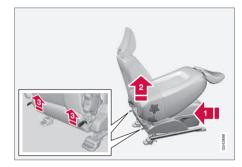
The front passenger seat backrest can be folded to a horizontal position to make room for a long load. Fold the backrest as follows:
