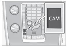
PAC is activated when the gear selector is moved to R if the system is selected in the MY CAR menu system or by pressing the CAM button in the center console. See My Car - introduction (p. 66) for a description of the menu system.
