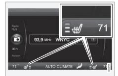
The current seat temperature setting is shown in the center console display
