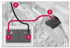
Connecting the jumper cables
