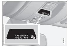
Occupant Weight Sensor (OWS) indicator light
