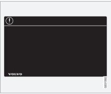
White ISO symbols and white text/image on a black or blue warning background and space for a message. If the information on decals of this type is ignored, damage to the vehicle could result.
