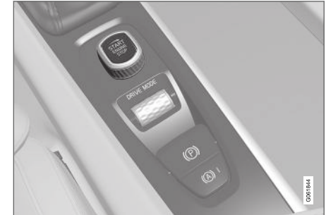
Start knob in the tunnel console.
