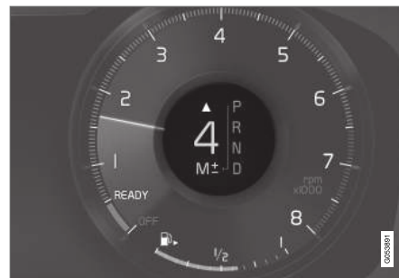
Gear shift indicator in the 12-inch driver display*.
