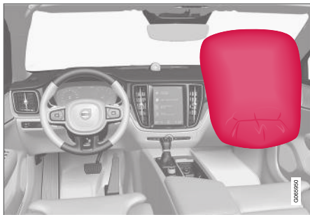
Front passenger airbag in front seat.
