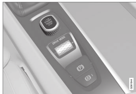
Start knob in the tunnel console.
