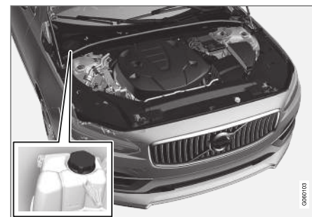
Coolant expansion tank, left-hand drive vehicle.
