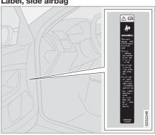
Location of decal for side passenger airbag, driver's side, front, left-hand drive car
