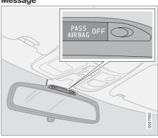
Indicator showing that the passenger airbag (SRS) is deactivated.
