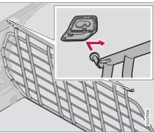
The protective grille in the cargo area prevents cargo or pets from being thrown forward in the passenger compartment in the event of heavy braking.
