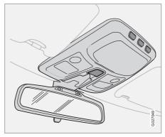
An acoustic signal and indicator lamp remind the driver and front seat passenger to use a seatbelt if either of them is not wearing one. The audio reminder is speed dependent (at low speeds), and time dependent (when the car is started). The visual reminder is located in the roof console and in the combined instrument panel.
