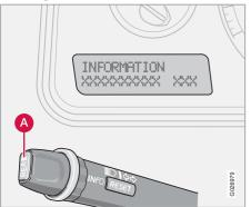
When a warning or indicator symbol illuminates, it is supplemented by a message appearing on the display.
