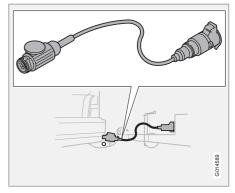
An adapter is required if the car's towing bracket has 13 pin electrics and the trailer has 7 pin electrics. Use an adapter cable approved by Volvo. Make sure the cable does not drag on the around.
