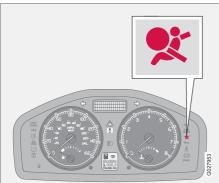
The airbag system<sup>1</sup> is continually monitored by the system's control module. The warning symbol in the combined instrument panel illuminates when the remote control key is turned to position **I**, **II** or **III**. The symbol goes out after approx. 6 seconds provided the Airbag system<sup>1</sup> is fault-free.
