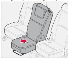
The centre seat in the second row can be slid farther forward than the other seats. Sliding the seat completely forward improves contact between a child sitting on the integrated booster cushion and front seat occupants.
