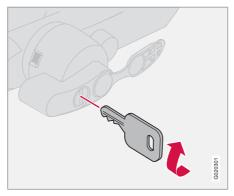
Ensure that the mechanism is in the unlocked position by turning the key clockwise.
