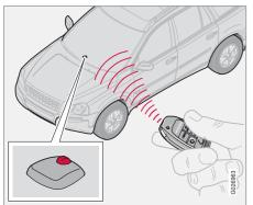
The remote control key locks/unlocks all side doors and the tailgate simultaneously. The side door lock buttons and inside handles are disengaged<sup>1</sup>.
