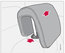
The centre seat head restraint can be adjusted to four different heights. Raise the head restraint as necessary.
