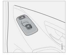
The control for the power window at the front passenger seat operates that window only.
