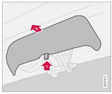
Remove the protective cover by first pressing in the catch and then pulling the cover straight back.
