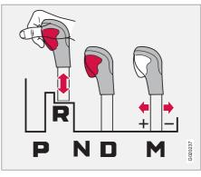
The gear selector can always be moved freely between  $\bf N$  and  $\bf D$ . Other positions are locked with a latch that is released with the inhibitor button on the gear selector.
