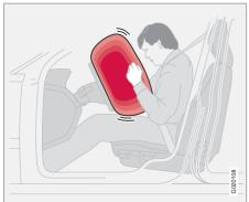
The car has an SRS airbag (Supplemental Restraint System) to supplement the protection afforded by the seatbelt on the driver's side. This airbag is fitted into the centre of the steering wheel. The steering wheel is marked SRS AIRBAG.
