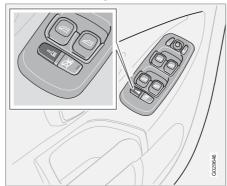
Automatic locking is activated and deactivated from the control panel in the driver's door. The function operates by locking the doors automatically when the speed of the car exceeds
