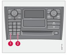
**AUTO** (1) seeks out the ten strongest radio stations and stores them automatically in a separate memory. The function is especially useful in areas where the radio stations and their frequencies are unfamiliar.
