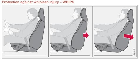
The whiplash protection system (WHIPS) consists of energy absorbing backrests and specially designed head restraints in the front seats. The system is actuated by a rear-end collision, where the angle and speed of the collision, and the nature of the colliding vehicle all have an influence.
