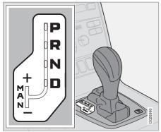
To move from the automatic driving position **D** to a manual position, move the gear selector to position **M**. To go from position **M** to the automatic driving position **D**, move the selector to position **D**.
