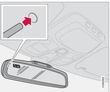
The upper left-hand corner of the rearview mirror has an integrated display that shows the compass direction in which the front of the car is pointing. Eight different directions are shown with English abbreviations: N (north), NE (north east), E (east), SE (south east), S (south), SW (south west), W (west) and NW (north west).
