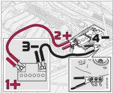
If the battery in the car has become discharged, you can "borrow" electric current from either a separate battery or from another car. Always make sure the crocodile clips on the jump leads are attached securely to eliminate sparks during the start attempt.
