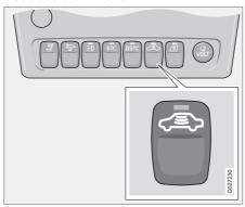
To avoid inadvertently triggering of the alarmfor example when leaving a dog in the car or during a ferry crossing - the movement and tilt detectors can be temporarily switched off.
