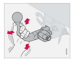
7. Check that the towball section is secure by pulling it up, down and back.
