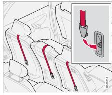
The car is equipped with mounting points for child seats. These mounting points are located on the rear of the rear seats.
