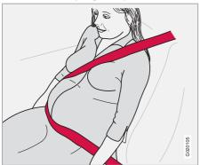
The seatbelt should always be worn during pregnancy. But it is crucial that it be worn in the correct way. The diagonal section should wrap over the shoulder then be routed between the breasts and to the side of the abdomen. The lap section should lay flat over the thighs and as low as possible under the abdomen. — It must never be allowed to ride upward. Remove all slack from the seatbelt and ensure that it fits close to the body. In addition, check that there are no twists in the seatbelt.
