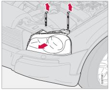
The entire lamp insert must first be removed when replacing dipped beam, main beam and parking lamp bulbs. To replace one of these bulbs, do the following and then consult the instructions for the specific lamp.
