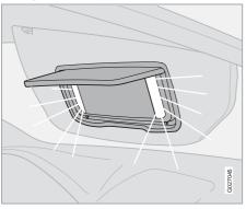
The light illuminates automatically when the cover is lifted.
