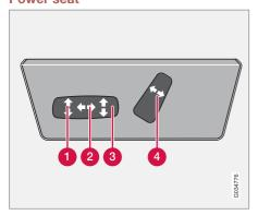
The seats can be adjusted for a certain time after unlocking the door with the remote control key without the key being inserted into the ignition switch. The seat can always be adjusted in ignition position I or II.
