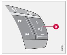
The four buttons at the bottom of the steering wheel keypad control both the radio and the phone. The function of the respective button depends on which system is active. The steering wheel keypad can be used to adjust volume, switch between preset stations and change CD tracks. The two upper buttons in the keypad (**Yes** and **No**) are used to answer and end phone calls respectively.
