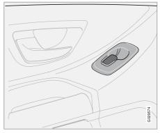
The rear door windows can be operated with the controls on the doors and the switch on the driver's door. If the light in the switch for blocking power windows in the rear doors (located in the driver's door control panel) is illuminated, the rear door windows can only be operated from the driver's door.
