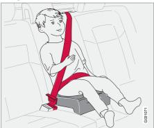
Volvo's integrated booster cushion for the centre rear seat is specially designed to provide optimum safety for children. Combined with the regular seatbelts the integrated booster cushion is approved for children weighing between 15 and 36 kg.
