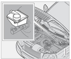
Brake and clutch fluid have a common reservoir1. The fluid level must be between the MIN and MAX marks. Check the level regularly. Change the brake fluid every other year or at every other regular service.
