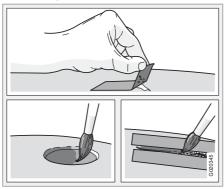
Before touching up paintwork, the car must be clean and dry and at a temperature above 15 °C.
