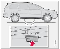
Remember to set out the warning triangle if you must change a wheel in a trafficked area. There are two jacking points on each side of the car. The jacking points are centred under the bottom of the doors.
