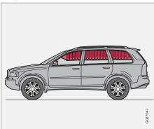
The inflatable curtain IC (Inflatable Curtain) is a supplement to the SIPS and the airbags. It is fitted in the headlining along both sides of the roof and protects all of the vehicle's outer seats. A sufficiently violent collision trips the sensors and the inflatable curtain is inflated. The inflatable curtain helps to prevent the driver and passengers from striking their heads on the inside of the car during a collision.
