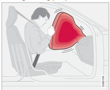
The car has an airbag to supplement the protection afforded by the seatbelt on the passenger side. This airbag is folded up into a compartment above the glovebox. The cover panel is marked **SRS AIRBAG**.
