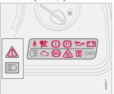
All indicator and warning symbols<sup>1</sup> illuminate when the remote control key is turned to position **II** before starting. This is to check that the symbols are working. When the engine starts, all the symbols should go out except the handbrake symbol, which only goes out when the brake is disengaged.
