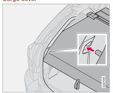
Pull out the cargo area cover, pull it over the cargo and hook it into the holes in the rear pillars of the cargo area.
