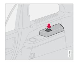
The digital TV box is located on the right-hand side of the cargo area
