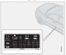
The tyre pressure label on the driver's side door pillar shows which pressures the tyres should have at different loads and speed conditions.
