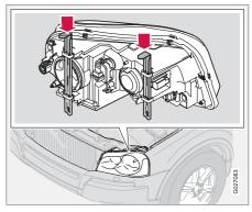
Refit the headlamp insert in reverse order. Check that the lock pins are correctly situated.
