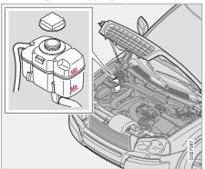
When topping up the coolant, follow the instructions on the packaging. It is important that the mixture of coolant concentrate and water is correct for the prevailing weather conditions. Never top up with water only. The risk of freezing increases with both too little and too much coolant concentrate.
