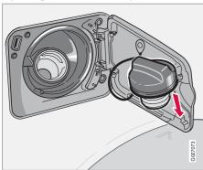
The fuel filler cap is inside the fuel filler flap on the right-hand rear wing and hangs up on the inside of the fuel filler flap.
