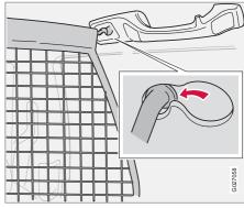
The safety net prevents luggage and cargo from being thrown forward in the passenger compartment during heavy braking.
