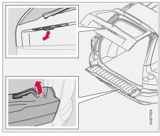
Open the tailgate by pulling the handle indicated in the illustration. Fold down the rear flap by lifting the handle up.
