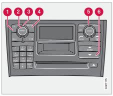
Press the **POWER** button **2** to switch the audio system on or off.
