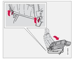
The passenger seat backrest can be folded forward to make room for long loads.
