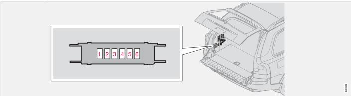
The fuse box is located behind the cover panel on the left-hand side.
