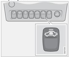
If someone is going to stay in the car but the doors must be locked from the outside, then the deadlocks function can be temporarily switched off.
