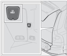
Slide down the cover when you wish to use the socket. It works regardless of whether the ignition is on or off.
