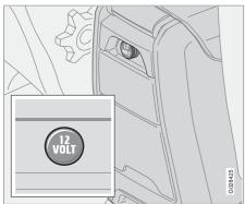
The electrical socket can be used for various accessories, such as mobile phone chargers and coolers. It is designed for 12 V. The maximum current is 10 A. For the socket to supply current, the remote control key must be in at least position I.
