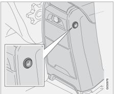
Button for rear seat heating, On/Off.
