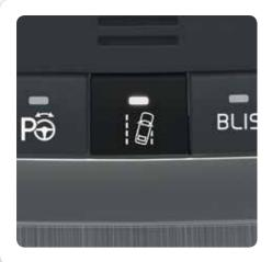
If the vehicle crosses a side marker line or the road's center dividing line, LKA will provide active steering assistance to help steer it back into the lane.
