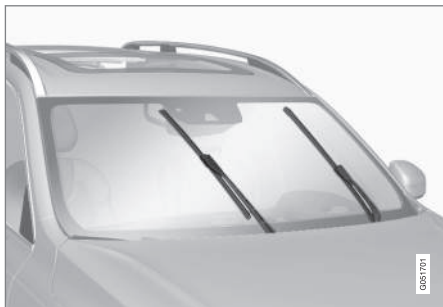
Viskerblade i servicestilling.
