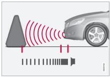
The distance monitored in front of the vehicle is approximately 2.5 ft (0.8 m). The audible signal comes from the audio system's front speakers.
