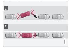
After the vehicle has backed into the parking space, its position in the space has to be adjusted by driving slightly forward and backing up.
