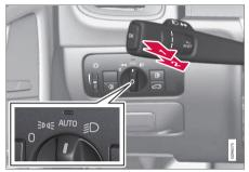
Headlight switch and steering wheel lever
