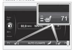
The current seat temperature setting is shown in the center console display
