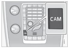
PAC is activated when the gear selector is moved to **R** if the system is selected in the **MY CAR** menu system or by pressing the **CAM** button in the center console. See My Car – introduction (p. 71) for a description of the menu system.
