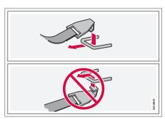
Fasten the attachment correctly to the ISOFIX/LATCH lower anchors
