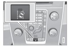
LKA can be switched on or off by pressing the button on the center console. A light in the button illuminates when the function is on.
