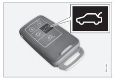
Trunk unlock button on the remote key
