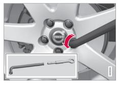
6. With the vehicle still on the ground, remove the plastic covers on the wheel nuts with the tool provided and use the lug wrench/towing eyelet to loosen the wheel nuts ½ – 1 turn by exerting downward (counterclockwise) pressure.
