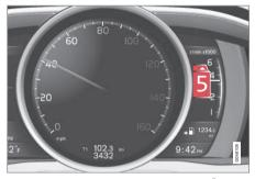
Gear shift indicator in a digital instrument panel\*6
