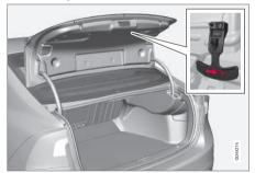
The vehicle is equipped with a florescent handle on the inside of the trunk lid, which can be used in an emergency situation to open the trunk from the inside. Pull the handle down to release the trunk lid. After use, the handle must be pushed back into its original position before the trunk can be closed.
