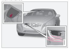
Camera and radar sensor<sup>6</sup>.
