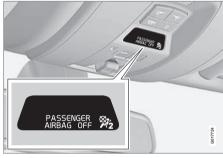
Occupant Weight Sensor (OWS) indicator light
