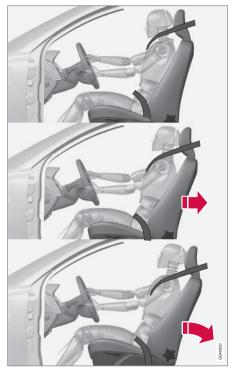
In the event of a rear-end collision, the hinges and brackets of the front seat backrests are designed to change position slightly to allow the
