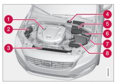
Engine compartment - 4-cylinder engines only
