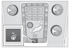
Button for steering wheel heating
