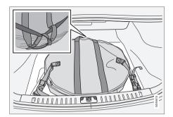
Turn the handle on the spare wheel bag in toward the rear seat. Secure the stitched strap hooks in the loading eyelets. Secure the long strap in one of the loading eyelets, wrap the strap around the spare wheel and through the lower handle. Secure the short strap on the long strap. Secure in the other loading eyelet and tighten.
