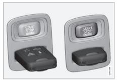
Ignition slot with remote key inserted (see Ignition modes (p. 74) for more information on ignition modes)
