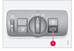
Press the button on the lighting panel (1) to unlock and pop open the trunk
