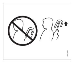
The center head restraint should be adjusted according to the passenger's height. The restraint should be carefully adjusted to support the occupant's head.
