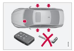
Locking/unlocking points with valet locking activated
