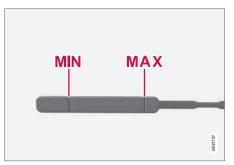
The oil level must be between the  $\boldsymbol{\mathsf{MIN}}$  and  $\boldsymbol{\mathsf{MAX}}$  marks on the dipstick
