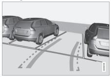
The lines on the screen are projected as if they were a path on the ground behind the vehicle and are directly affected by the way in which the steering wheel is turned. This enables the driver to see path the vehicle will take, even if he/she turns the steering wheel while backing up.
