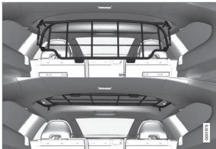
Your vehicle can be equipped with a steel grid that helps prevent objects in the cargo area from moving forward into the passenger compartment.
