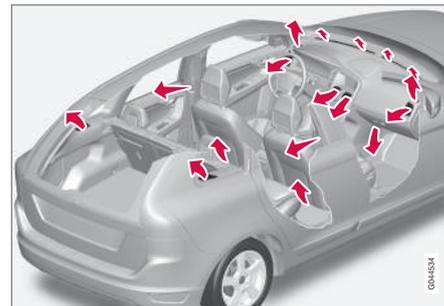
The incoming air is distributed from a number of different vents in the passenger compartment.
