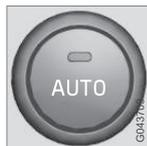
The function automatically regulates cooling, heating, blower speed, recirculation, and air distribution to maintain the chosen temperature. If you select one or more manual functions, the other functions continue to be controlled automatically. The air quality sensor is engaged and all manual settings are switched off when **AUTO** is pressed. The display shows **AUTO CLIMATE**.
