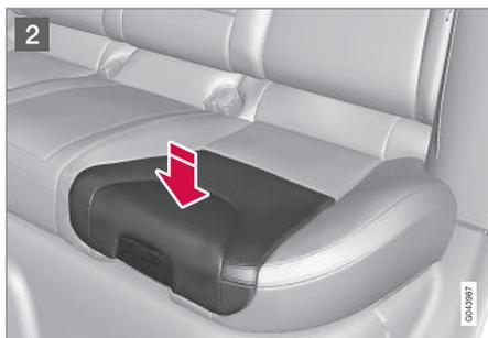
The booster cushion can be folded down completely (stowed) from either the stage 1 or stage 2 positions.
