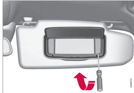
1. Insert a flat screwdriver under the glass and carefully exert upward pressure to release the retaining lugs.
