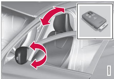
Each remote key has a feature that enables it to store (remember) the position of the power driver's seat and door mirrors when the vehicle is locked with that remote key.
