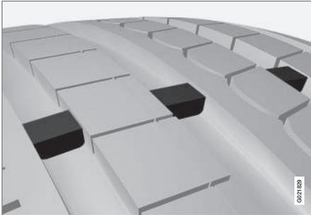
The tires have wear indicator strips running across or parallel to the tread. The letters **TWI** are printed on the side of the tire. When approximately 1/16" (1.6 mm) is left on the tread, these strips become visible and indicate that the tire should be replaced. Tires
