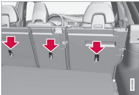
Your Volvo is equipped with child restraint top tether anchorages in the rear seat. They are located on the rear side of the backrests.
