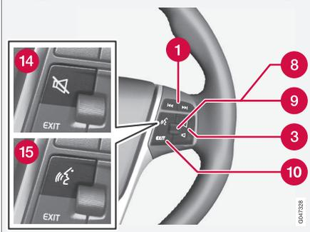
Corresponding controls - steering wheel keypad and center console
