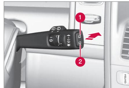
Move the lever forward to start the tailgate washer.
