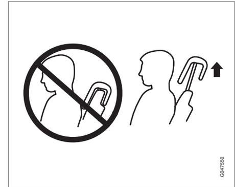
The center head restraint should be adjusted according to the passenger's height. The restraint should be carefully adjusted to support the occupant's head.
