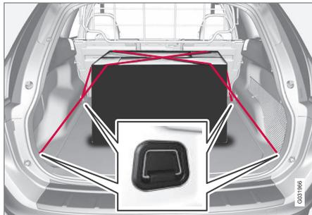
The load anchoring eyelets on both sides of the vehicle are used to fasten straps, etc., to help anchor items in the cargo area.
