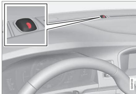
The status of the alarm system is indicated by the red indicator light on the dashboard (see illustration):
