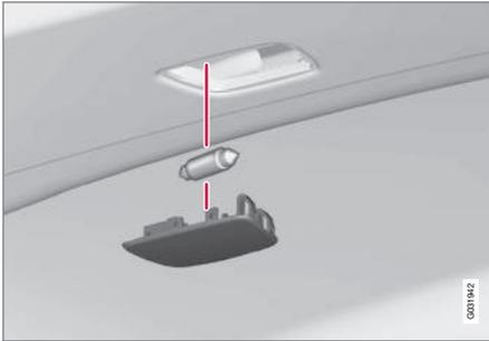
1. Insert a screwdriver and gently turn so that the bulb housing comes loose.
