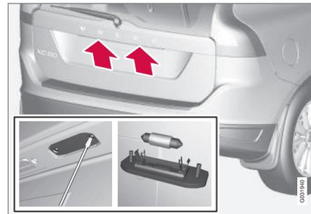
1. Remove the screws with a screwdriver.
