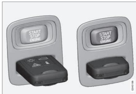
2. Insert the remote key into the ignition slot (also on vehicles with the optional keyless drive). This will turn off the alarm.
