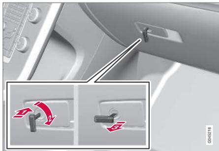
The glove compartment can only be locked and unlocked using the detachable key blade in the remote key. See page 64 for information on removing the key blade from the remote key.
