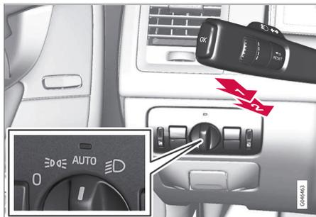
Headlight switch and steering wheel lever
