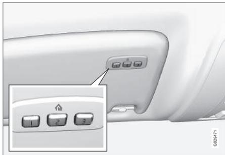
The HomeLink<sup>1</sup> Wireless Control System provides a convenient way to replace up to three hand-held radio-frequency (RF) transmitters used to activate devices such as gate operators, garage door openers, entry door locks, security systems, even home lighting. Additional HomeLink information can be found on the Internet at [www.homelink.com](http://www.homelink.com) or by phoning the hotline at 1-800-355-3515.
