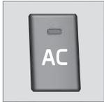
When the indicator light in the button is on, the air conditioning is controlled automatically. This cools/heats and dehumidifies the incoming air. When the indicator light in the button is off, the
