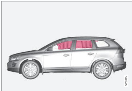
This system consists of inflatable curtains located along the sides of the roof liners, stretching from the center of both front side windows to the rear edge of the rear side door windows. It is designed to help protect the heads of the occupants of the front seats and the occupant of the outboard rear seating positions in certain side impact collisions.
