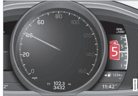
*Gear shift indicator in a digital instrument panel\*<sup>1</sup>*
