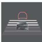
Five different time intervals can be selected and are shown in the display as 1–5 horizontal bars. The greater the number of bars, the longer the time interval. One bar represents approximately
