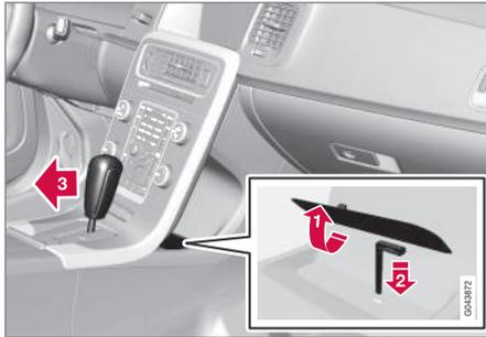
If the vehicle cannot be driven, for example because of a dead battery, the gear selector must be moved from the **P** position before the vehicle can be moved<sup>3</sup>.
