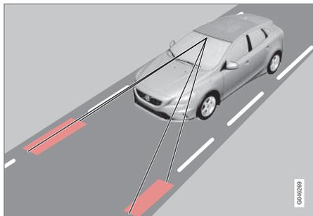
This function is designed to help reduce the risk of accidents in situations where the vehicle leaves its lane and there is a risk of driving off the road or into the opposite lane. LDW consists of a camera that monitors the lane's side marker lines. The driver is alerted by an audible signal if the vehicle crosses a side marker line or the road's center dividing line.
