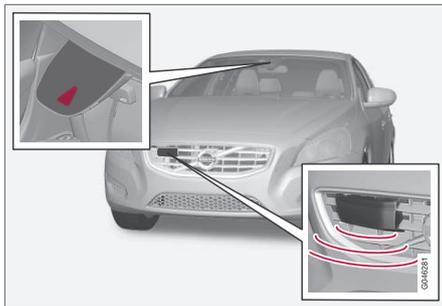
Camera and radar sensor<sup>1</sup>.
