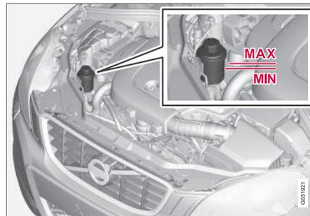
Check the level frequently. The fluid does not require changing. The fluid level must be between the **MIN** and **MAX** marks. For capacities and recommended fluid grade, see page 372.
