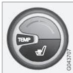
Press the lower section of the button repeatedly until the desired number of indicator lights illuminate:
