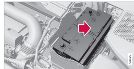
2. Move the battery inward and to the side until it reaches the rear edge of the box.
