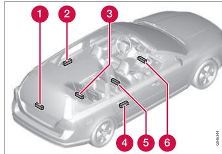
The keyless drive system has a number of antennas located at various points in the vehicle.
