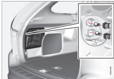
The brake lights and taillights are replaced from inside the cargo area.
