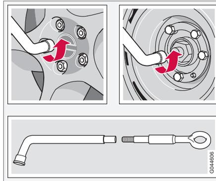
6. With the vehicle still on the ground, use the lug wrench/towing eyelet to loosen the wheel nuts  $\frac{1}{2}$  – 1 turn by exerting downward (counterclockwise) pressure.
