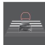
Different time intervals can be selected and are shown in the instrument panel<sup>3</sup> as 1–5 horizontal bars. The greater the number of bars, the longer the time interval. One bar represents a time interval of approximately 1 second; 5 bars is approximately 3 seconds.
