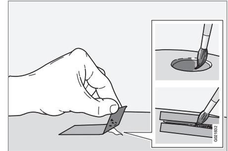
1. Place a strip of masking tape over the damaged surface. Pull the tape off so that any loose flakes of paint adhere to it.
