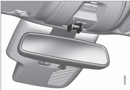
Both the laminated panoramic roof and the sun shade are operated by the controls in the ceiling console, near the rear-view mirror. The vehicle's ignition must be in mode **I** or **II** before the laminated panoramic roof/sun shade can be operated.
