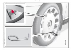
5. Screw together the towing eye with the wheel wrench\* to the stop position.
