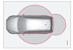
The red rings in the above figure indicate the range covered by the system's antennas.
