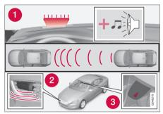
Collision warning system warning lamp and warning sound<sup>6</sup>.
