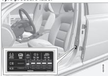
The tyre pressure label on the driver's side door pillar (between frame and rear door) shows which pressures the tyres should have at different loads and speed conditions. This is also specified in the tyre pressure table, see Tyres - approved tyre pressures (p. 425).
