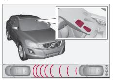
Laser sensor transmitter and receiver window 13.
