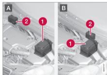
A: Left-hand drive car. B: Right-hand drive car. (1) Starter battery<sup>17</sup> (2) Support battery.
