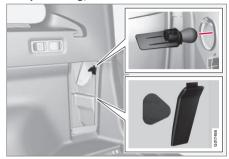
The direction indictor bulb in the rear lamp cluster is replaced from inside the cargo area.
