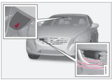
Camera and radar sensor<sup>25</sup>.
