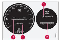
Message and graphic in the display. The lefthand display is shown in the digital combined instrument panel and the right-hand in the analoque.
