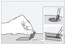
Before work is started, the car must be clean and dry as well as at a temperature above 15 °C.
