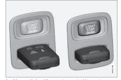
Ignition switch with remote control key extracted/inserted.
