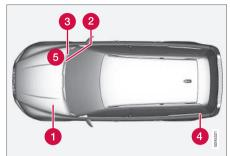
Central electrical unit locations in a left-hand drive car. In a right-hand drive car the central electrical units under the glovebox change sides.
