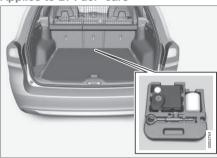
The emergency puncture repair kit is located in the storage compartment in the front part of the cargo area.
