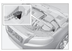
Topping up the washer fluid takes place by opening the blue cap.
