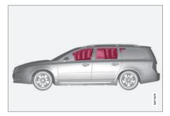
Inflatable curtain IC (Inflatable Curtain) is part of the SIPS system (p. 36) and the airbag system (p. 31). It is fitted along both sides of the headlining and helps protect the driver and passengers in the car's outer seats. A sufficiently violent collision trips the sensors and the inflatable curtain is inflated.
